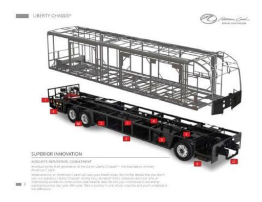
Figure: This is an example of the substructure in a diesel pusher. (Copied from a Liberty Chassis/American Coach brochure available online and during the tour.)
