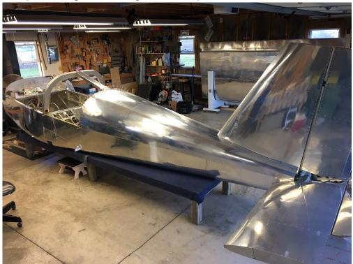
So far the empennage/tail kit, wing kit and fuselage kit are complete. Currently, Team Stark is working on the finish kit to add the cowling, engine mount, canopy, wheels, brakes, nose gear components, wiring harness and fuel tank components. Once that is done, the next steps are the avionics and then the Rotax engine with a composite ground-adjustable propeller.
