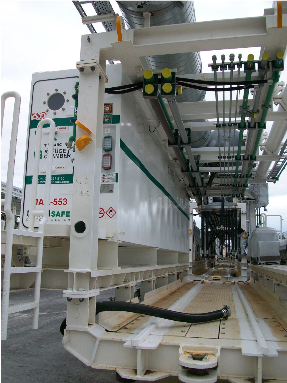
This picture shows four sections lined up as they will appear underground. Note light
