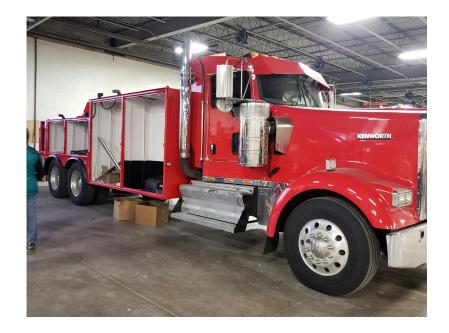
In addition to cranes, already mentioned, SST installs lighting, power supplies, compressors, shelving, and more. There were scores of details such as blowers to pressurize cabinets for the exclusion of off-roading dust.
