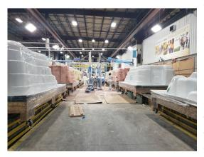
The tub then enters a large room with a cutoff saw and a lot of dust collection. The saw will remove the rough top edge of the saw and operators with respirators and air breathing devices will drill the holes for the jets. Upon exit, a team will begin to plumb the water and airlines as well as install all the jets and pumps. The wood framing is then assembled around the tub and it is prepared to be flipped
