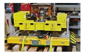
reminiscent of warehouse donkeys but far less vulnerable to disruptions on factory floors shared with humans. These E-Carts (electronic carts) can move assemblies along a line, rotate assemblies, with the intent to be robotically loaded and unloaded. The E-Carts and robotics combination allows a range of work at different stations along an assembly line.
